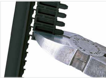
Remove unrequired areas from the sidewalls.
