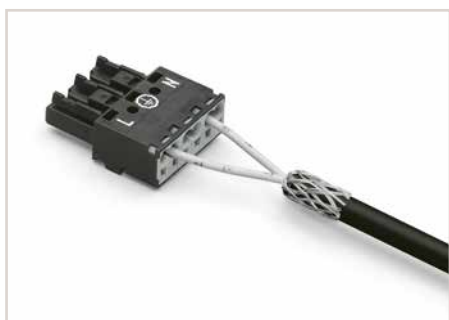
Apply the shield to the rubber cable. Strip length, outer insulation = 55 mm Shield length = 10 mm
