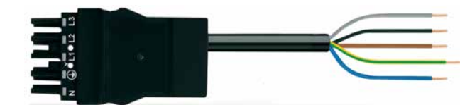
Connecting cable ► Socket - free end ► Strip length (outer insulation): 55 mm
